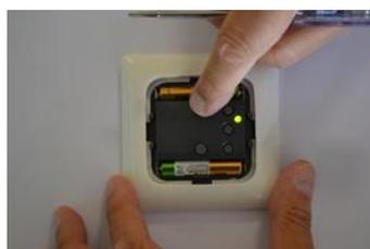
4. Get the Z-Wave® device you want to control to issue a Node Information Frame (generally done by pressing once or several times on a **FUNCTION (inclusion/exclusion) button** on the device – see manual of the device
