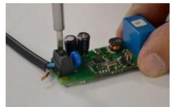
**WARNING:** If you reverse the mounting direction of the wires, your Swiid® cord switch will not work at all. This will not damage your Swiid® cord switch, but you will need to reinstall the wires all over again always taking care to disconnect the electrical power cord.
