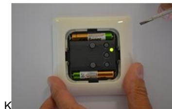
If you are **not** successful, the LED on the wall controller switch continue blinking **green** for around 5 seconds before turning **red** for 1-2 seconds.
