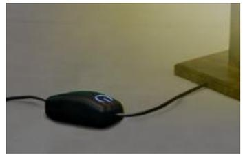
**WARNING:** The presence near your Swiid® cord switch of grounded metallic objects or of high power conductors can affect the Z-Wave® radio signals and thus the remote controlling of your Swiid® cord switch.
