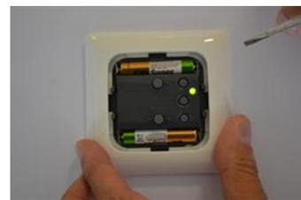
If you are **not** successful, the LED on the wall controller switch continue blinking **green** for around 5 seconds before turning **red** for 1-2 seconds.
