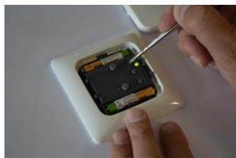
3. **Single click (or double click)** on either the **UP** or the **DOWN** button the front of your wall controller switch. The LED on the wall controller switch will **blink green** to indicate it is ready to associate a device
