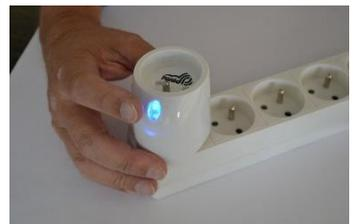
3. The inclusion/exclusion process should then start automatically and the LED will remain lit **blue** or **yellow** based on switch status. This indicates that the Z-Wave® inclusion/exclusion process was successful.
